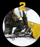
Attach the winch cable to the plow using a guiding hook/roller.
